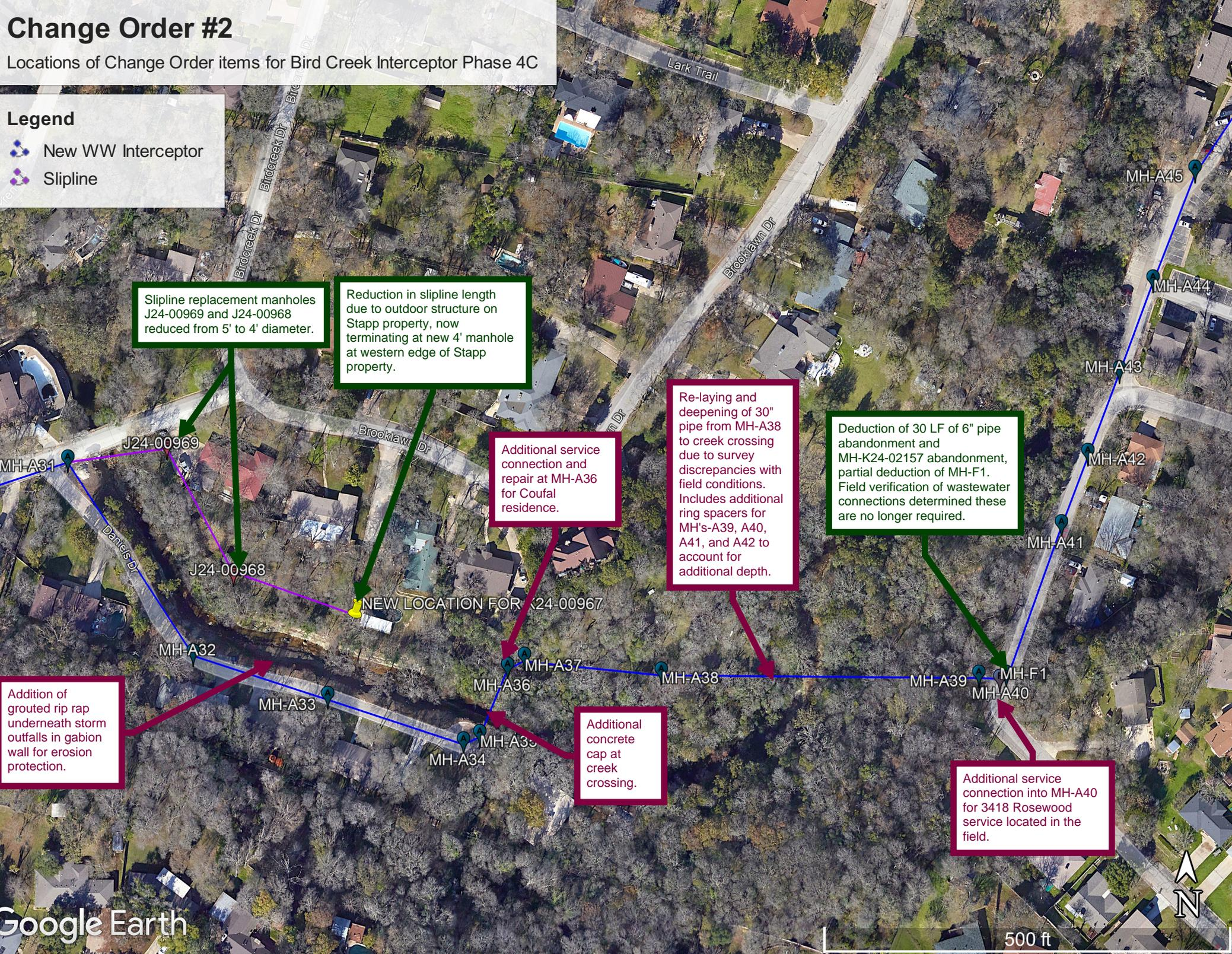
Slipline replacement manholes J24-00969 and J24-00968 reduced from 5' to 4' diameter.
